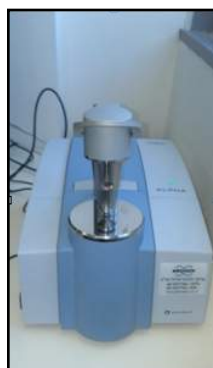
Figure 1: BRUKER FTIR spectrometer used in our analysis
